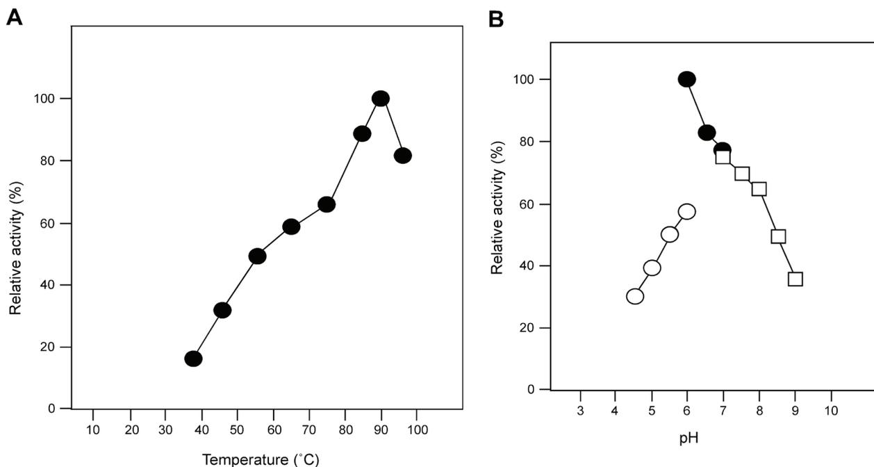
**Fig. 4.** Effect of temperature and pH on TK1111 enzyme activity. A) Optimal temperature of the enzyme activity. Assays were performed at various temperatures ranging from 37 to 95 °C under standard conditions. B) Optimal pH for TK1111 enzyme activity. Assays were conducted in various buffers at 50 °C. Buffers used were: acetate buffer, open circles; phosphate buffer, closed circles; Tris-Cl buffer, open squares.
